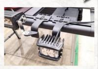
This universal mounting kit allows the fitment of 4 spotlights, a light bar or combination of both if required. Ideal for aluminium roof racks with a T slot system or any flat surface.
