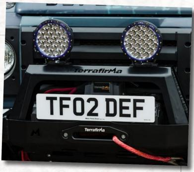
The brightness and light penetration is incredible. The aluminium mounting brackets are vibration resistant and allow for a large range of adjustment. A comprehensive wiring harness & switch and 3 sets of bezels in red, blue and amber are included with each set.
