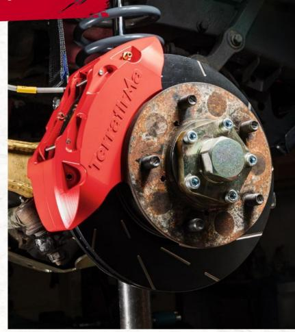
Terrafirma performance brake upgrade kits include huge 6 piston front calipers, EBC Redstuff brake pads with increased surface area and extra-large 330x 32mm vented and grooved brake discs, larger 4 piston rear calipers again with EBC Redstuff brake pads.
