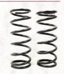
medium load front springs. Avoid fitting these springs if you are not carrying the load as the lift may be too great and could cause over extension of the rear shocks.
