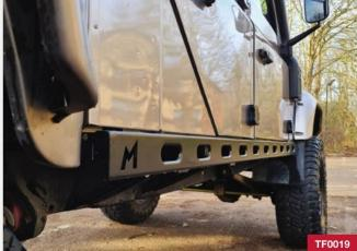
Terrafirma Skeleton rock sliders for Defenders are made from 3mm mild steel with punched and swaged slotted holes for weight reduction and unique styling, finished in satin black powder coat these rock sliders are chassis mounted and fully adjustable to ensure the perfect fit.
