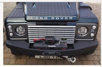
With these bumpers the winch is raised above the chassis rails and with tapered and swept back wings approach angle and styling are optimised even with the air-conditioned Defender versions. The Terrafirma Pro Taper bumpers are available to suit both the conventional 'small chassis' winches with pulling capacities up to 12000lbs as well as the 'Bigger is Better' super
