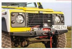
user looking for a winch mount with additional protection, ideal for builders, tree surgeons and farmers etc. Commercial bumpers are made from 5mm steel and are very strong in their construction. Each bumper incorporates 2 jacking points that will accept the standard jack or a Hi-lift jack adaptor as well as 2 recovery points and have tapered ends for a touch of style.
