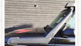
**TF1039** is specifically for the Discovery 2 V8 petrol and Td5 and is supplied as a 3 piece high grade moulded plastic unit mounted to the LH wing and A post.
