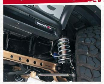
Monotube shocks perform at a higher level utilising a floating piston to completely separate the high-pressure nitrogen from premium grade suspension fluid that eliminates aeration. The high gas pressure allows for more responsive valving which increases performance when its needed most, resulting
