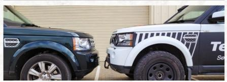
Standard height vehicle vs vehicle fitted with conversion kit TF266
