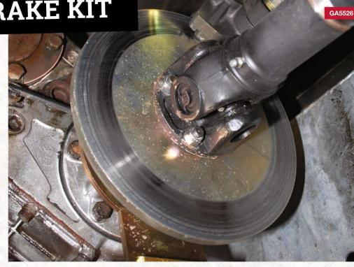
become partially or even completely seized. A seized brake is almost as likely to seize on as it is off which can then lead to vibration, overheating and accelerated wear. All these issues ultimately result in a handbrake that does not work.
